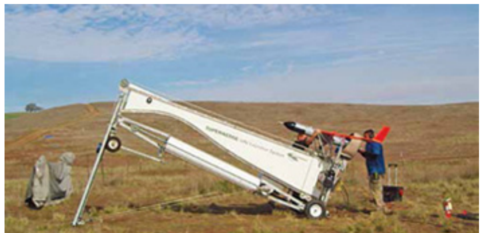
The catapult-launched ScanEagle is a larger model of an unmanned aircraft system. Photo by Keith Cunningham
